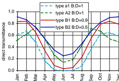
Fig. 5: Monthly direct solar transmittance of different shading metal grids
