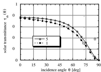
Fig. 2: Characteristic solar transmittance for 50 and 100mm honeycomb layer between two glass sheets;  $U=1.3$  W/m<sup>2</sup>K and 0.9 W/m<sup>2</sup>K (estimated from literature data)
