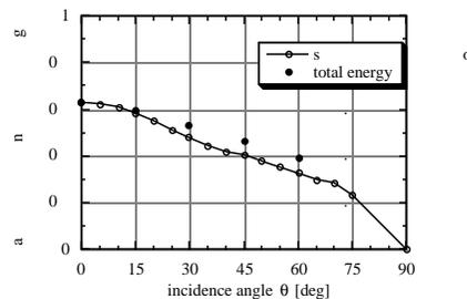
Fig. 4: Transmittance of 100mm StoTherm-Element (total solar energy transmittance includes effect of absorber  $\alpha=95\%$ )
