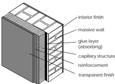
Fig. 3: Principle of StoTherm®
