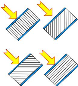
Fig. 1: Different orientations of the honeycomb layer within a LES glazing give flexibility for the application e.g. in roof-lights and sheds
