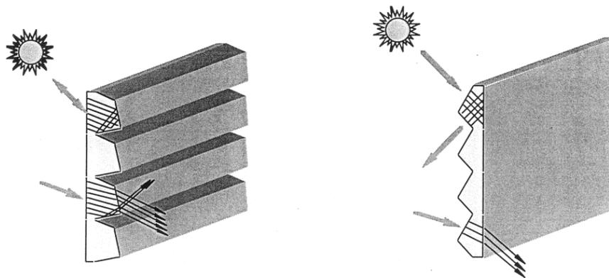
Figure 3: Tilted prismatic and saw-tooth type
