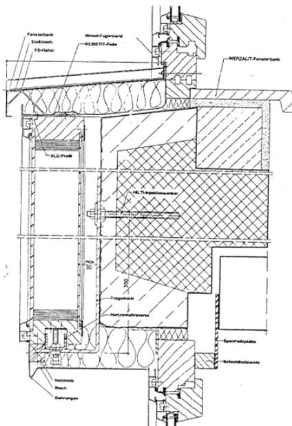
Figure 1: Sketch of improved construction including window detail
