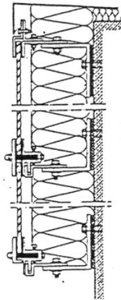
Figure 2: Opratrec system construction
